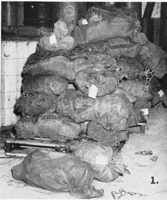
Cast iron sprinkler bases are delivered to our Receiving Room in burlap bags (photo No. 1). Note the untidy appearance. Oftentimes, jitneys hit the bags, knocking off and breaking the pieces.
